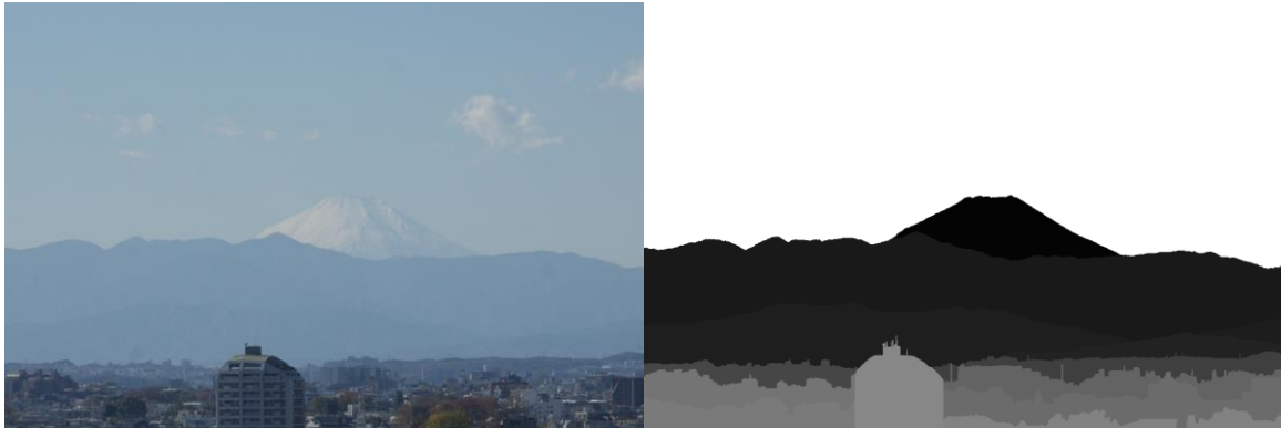
Figure 3.9. Left: Real scene of Tokyo city (Atmospheric turbidity was estimated as T=1.9 ) captured by Canon EOS5D. Right: The corresponding depth map.
