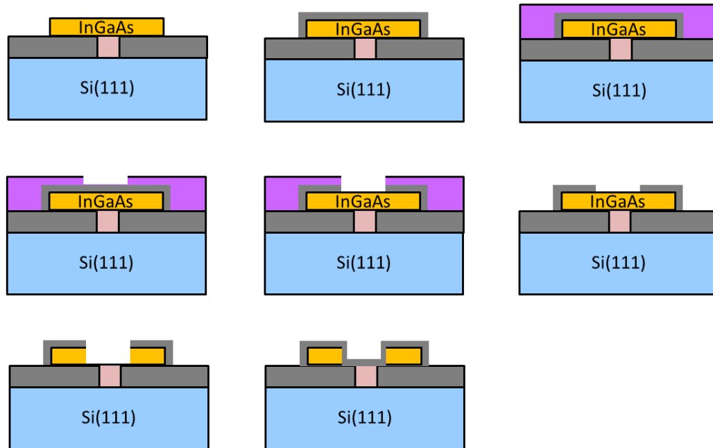
Fig. 4-1 Process flow of hollow hexagonal InGaAs cavity on Si.
