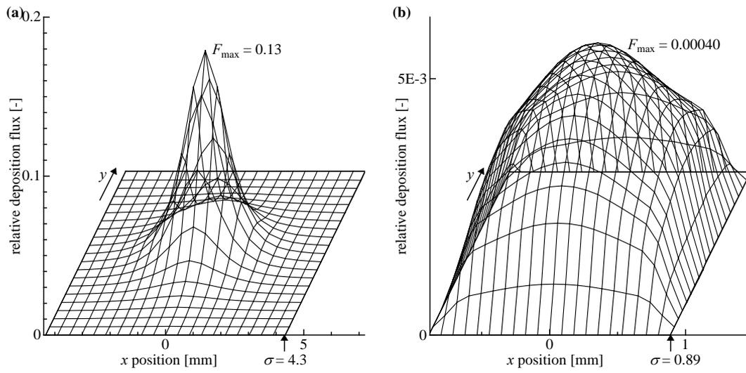
Figure 4. Spatial distributions of deposition flux calculated for  $t = 0.32$  mm,  $g = 1.0$  mm, and  $h =$  (a) 1.0 and (b) 0.050 mm.
