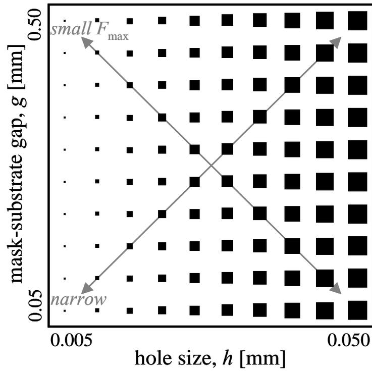
Figure 7. Example of the mask layout to produce a series of spatial distributions of deposit on a single substrate by using the CMD method.
