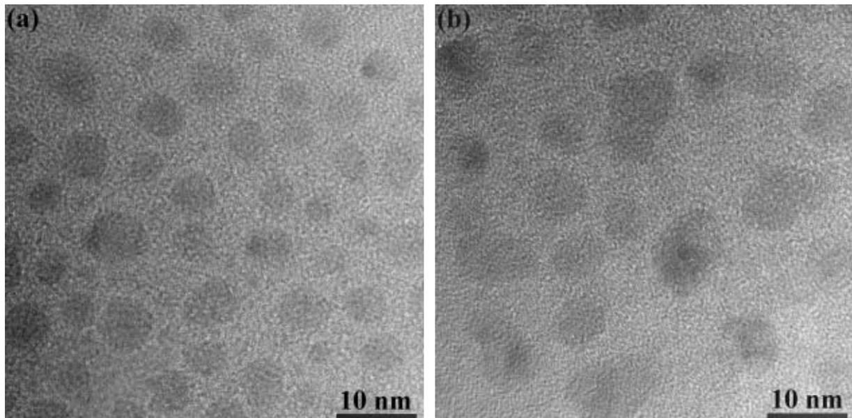
Figure 6. TEM images of Cu nanoparticles formed by sputter-deposition of Cu on SiO<sub>2</sub> substrates at a (a) high deposition flux of 0.80 nm/s for 25 s and (b) low deposition flux of 0.014nm/s for 140 s.
