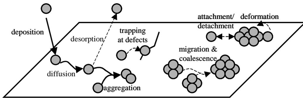
Figure 1. Schematic of nucleation and growth processes of nanoparticles on a substrate surface.
