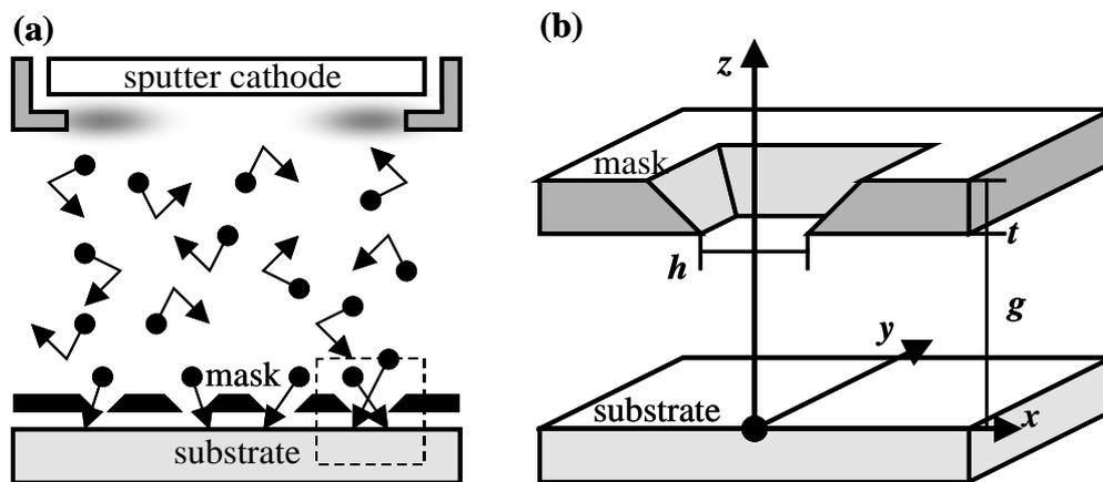
Figure 3. Schematic of the CMD method applied to a sputter-deposition system. (a) Entire sample and (b) a single hole. (b) is the enlargement of the dashed box in (a).
