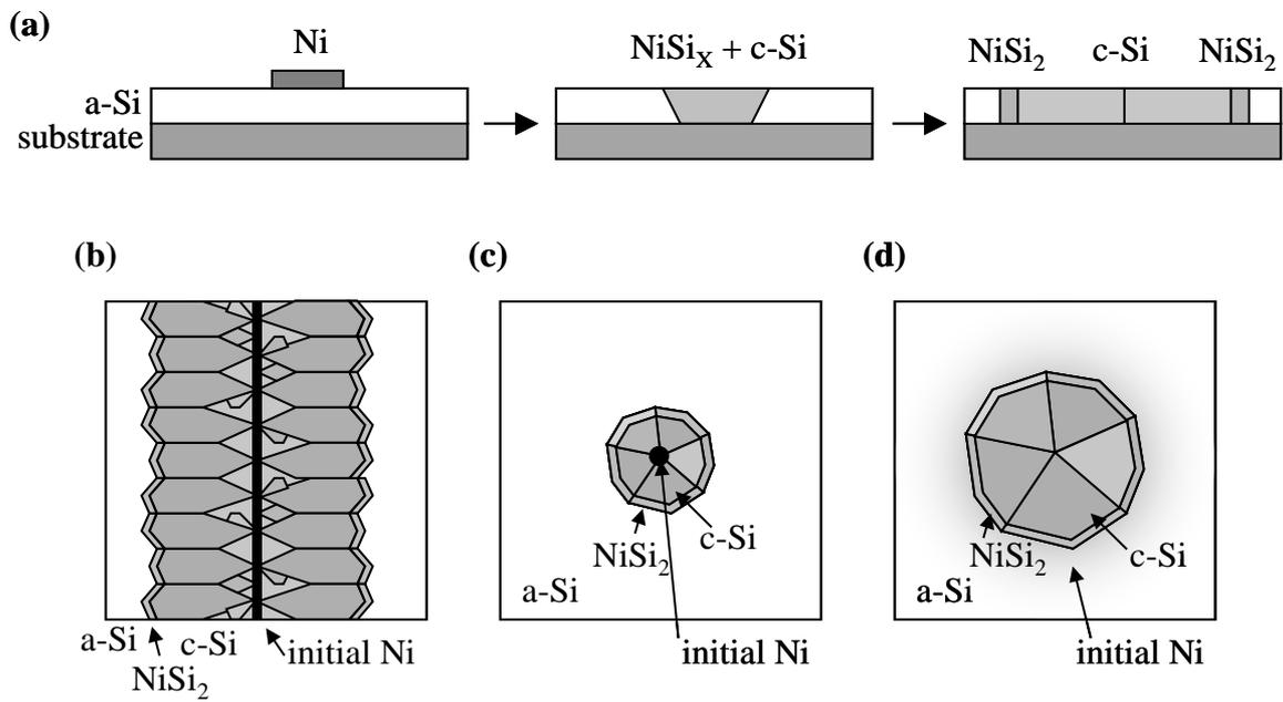
Figure 2. (a) Cross-sectional images of the phenomena occurring during Ni-MIC. Top view of the resulting structures after Ni-MIC with a (b) line pattern of Ni and (b) dot pattern of Ni. (d) A radial profile of Ni concentration applied to Ni-MIC, which might enhance MILC.
