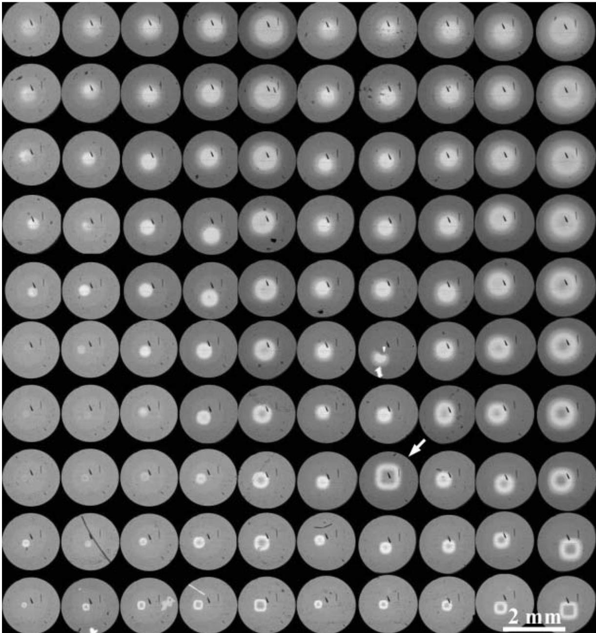
Figure 8. Optical microscopy images of a crystallized a-Si sample with 100 Ni patterns formed on a single sample by the CMD method. Each circle represents a single Ni pattern. Arrow indicates an irregularly large pattern caused by an irregularly large hole.
