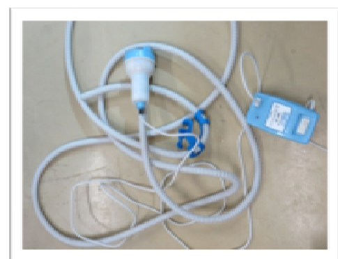
h. Water transfer pump.
