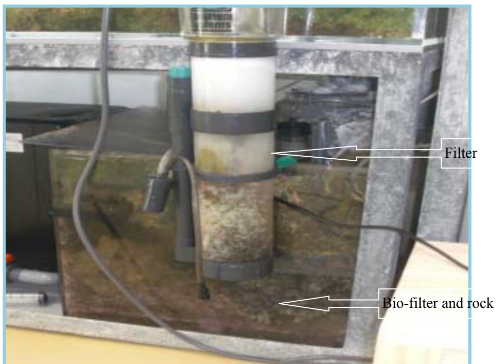
Fig 3.12 Water purifying unit of the tank system.
