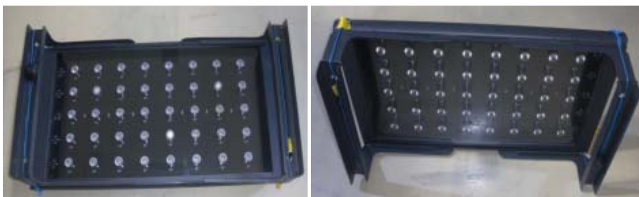
Fig 3.9 LED light used for Coral growth measurement.
