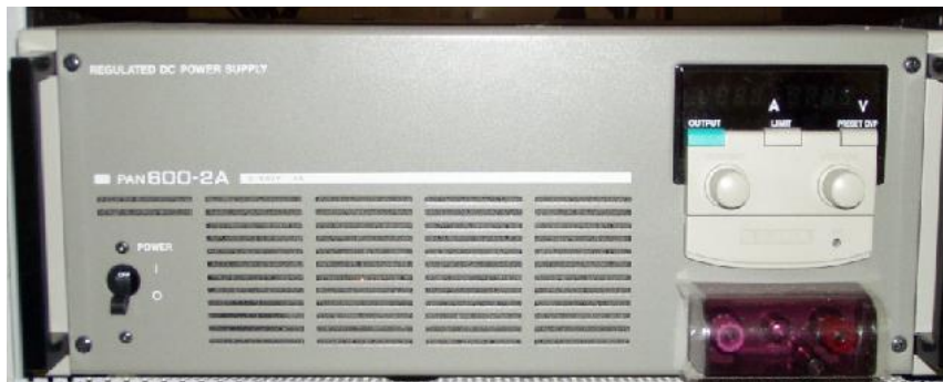
(e) Keeper of the cathode
