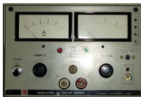
Figure 3.18 A power supply for the filament of an emissive probe.
