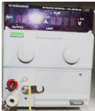
Figure 3.25 Power supply for single probe voltage biasing.
