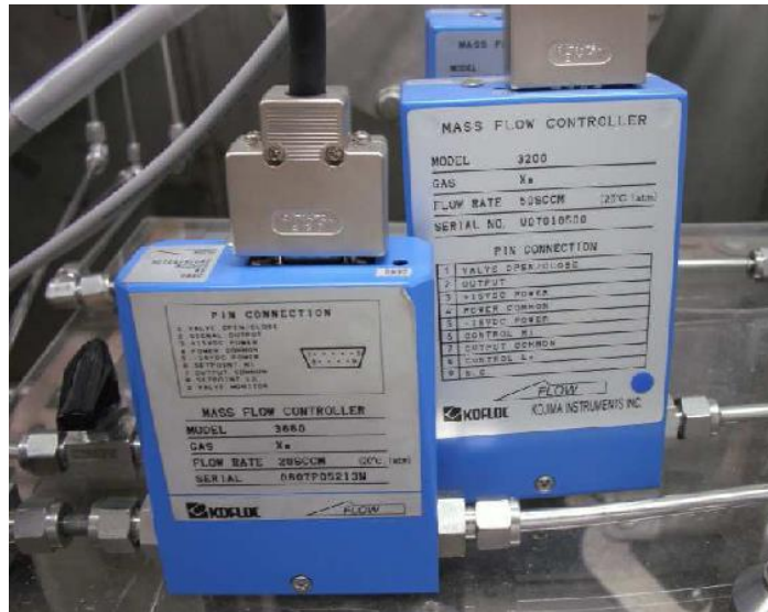
Figure 3.5 Mass flow controllers (Hongo)
