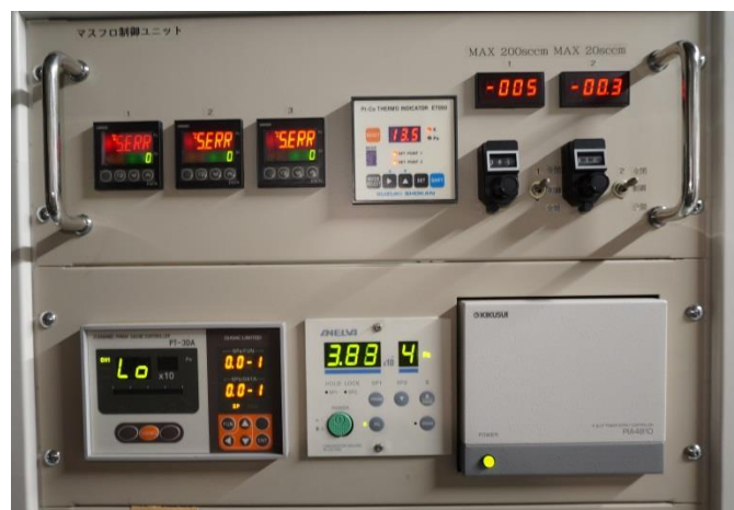
(c) A control unit with vacuum gauges and a thermometer
