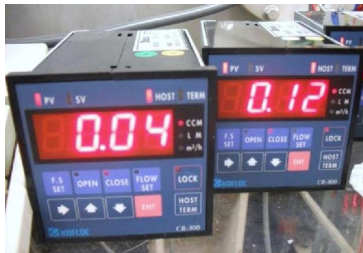
Figure 3.6 Read out units of the mass flow controllers (Hongo)
