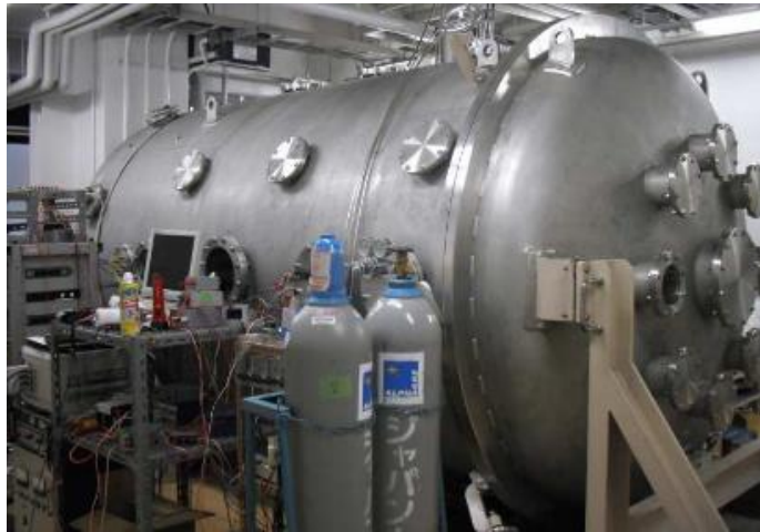
Figure 3.13 A large vacuum chamber (Hongo).
