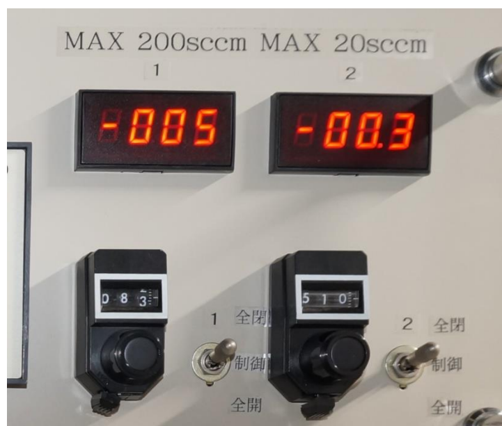
Figure 3.8 Read out units of the mass flow controllers (Kashiwa).
