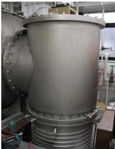
(a) An oil diffusion pump
