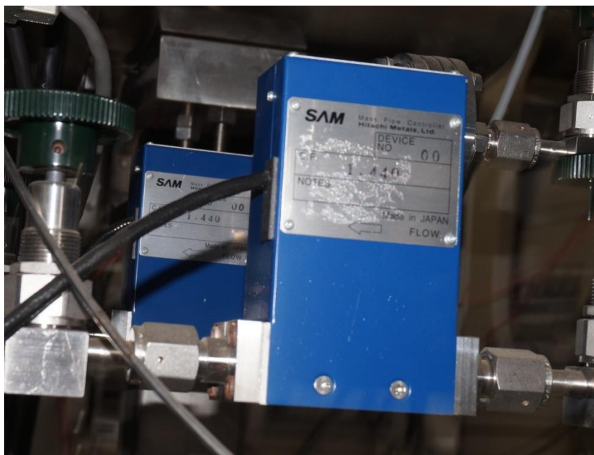
Figure 3.7 Mass flow controllers (Kashiwa).
