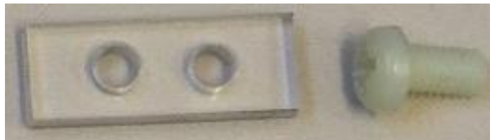
Figure 3.28. Reed Valve and Acrylic Window Attachment of Insulator
