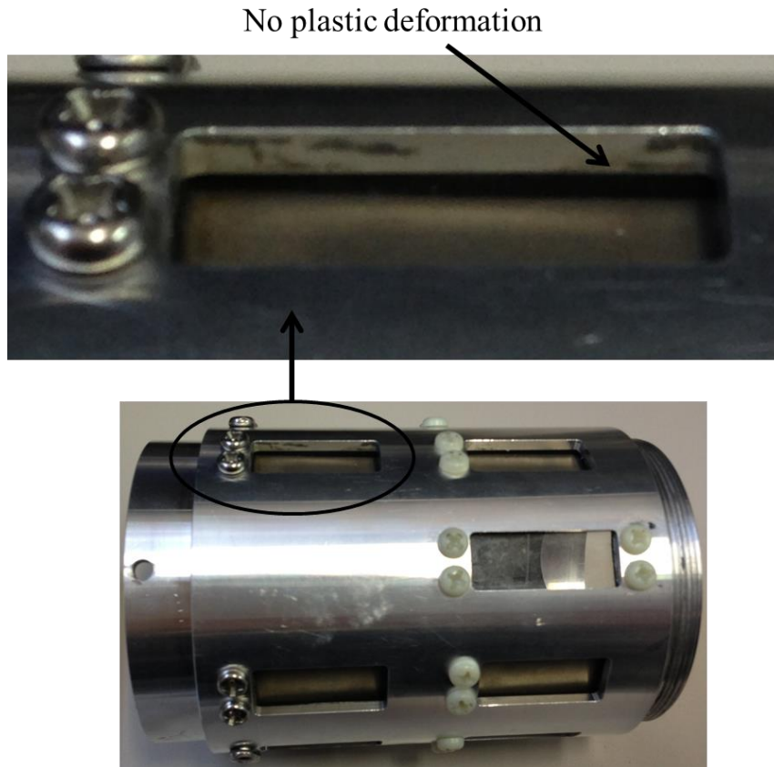
Figure 3.16. Reed Valve after the Experiment
