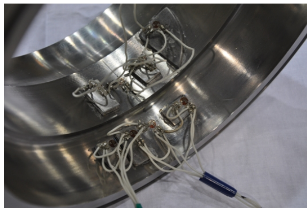
Fig. 4.10: Strain gage glued to inner surface of intersection.
