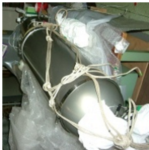
Fig. 1.2: Cylindrical pressure hull of TSUNASAND.
