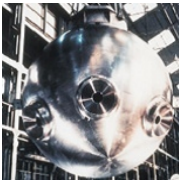
Fig. 1.1: Spherical pressure hull of SHINKAI6500.
