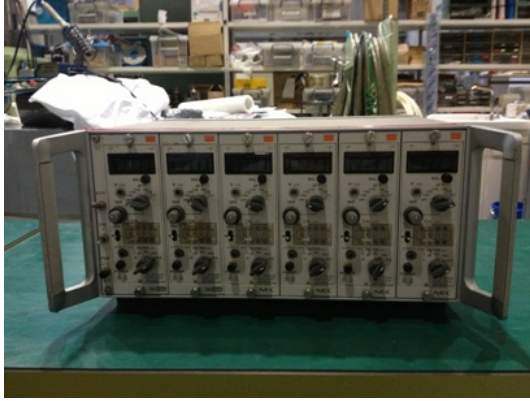
Fig. 4.13: Strain amplifier.
