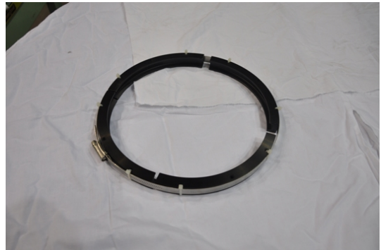
Fig. 4.8: V-Band made of Delrin .
