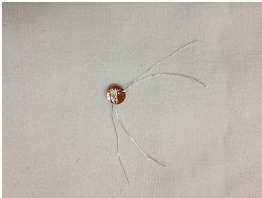
Fig. 4.14: Strain gage.
