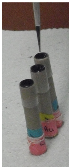
Fig. 1.2: Solid-contact ISEs. Carbon black is mixed into the ion-selective membranes.
