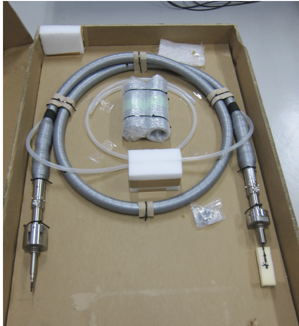
Fig. 3.18: 3000 m pressure-resistant laser delivery and plasma observation fiber cable used in the sea experiments.
