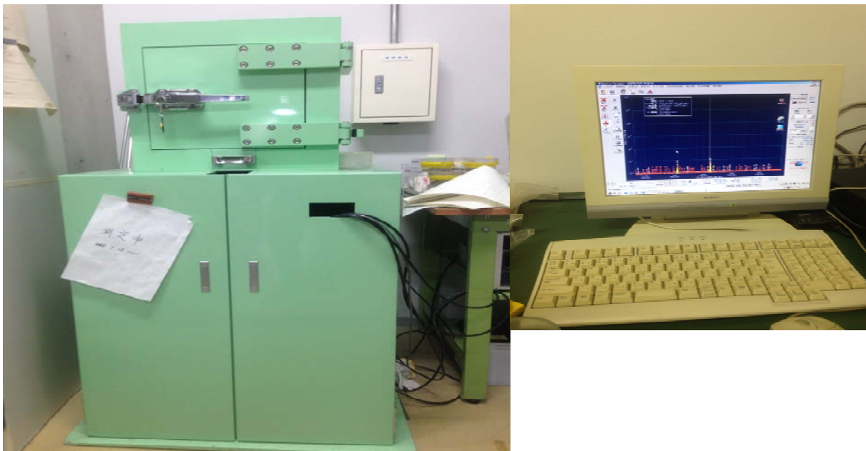
Figure 6 : EG & G ORTEC GAMMA-XR HPGe (High-purity Germanium) Coaxial Photon Detector
