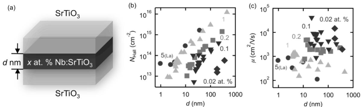
Fig. 1 (a) A schematic diagram of Nb  $\delta$ -doped SrTiO<sub>3</sub> heterostructures. (b) Sheet carrier density  $N_{\text{Hall}}$ , and (c) Hall mobility  $\mu$  estimated by the Hall measurement at temperature  $T = 2$  K.
