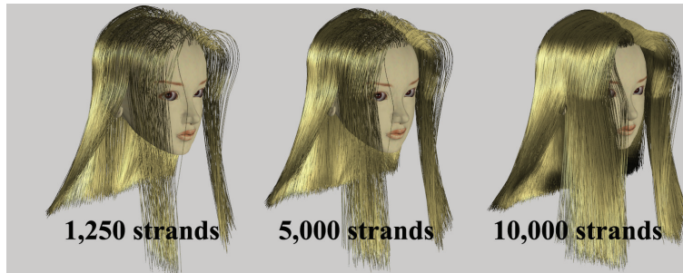
Figure 4.14: Increasing hair strands greatly improves the visual quality. From left to right, there are 1,250, 5,000 and 10,000 hair strands on the head.
