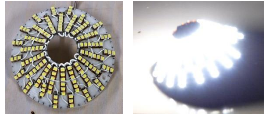
Figure 3: Handmade 162 LED's Array
