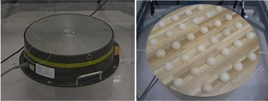
Fig. 2.4: The turntable (left) with fixed revolution speed and the test sample (right) setting on the turntable.
