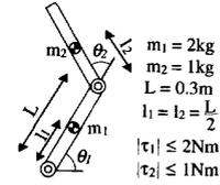
Fig. 2. Two-degree-of-freedom manipulator.
