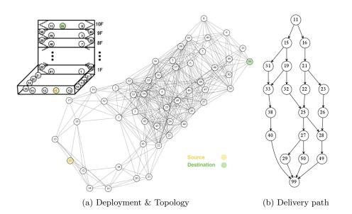
Figure 2.4: Deployment, topology and delivery path of the experimented network.
