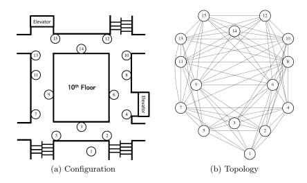
Figure 4.3: Deployment configuration and topology of the experimented network.
