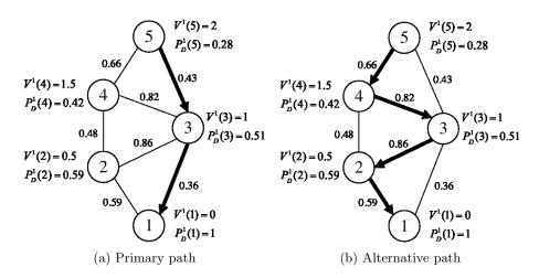
Figure 3.6: The example of primary path and alternative path from node 5 to node 1.
