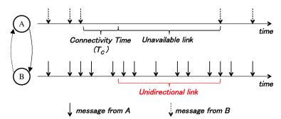
Figure 3.3: Example of the unidirectional link between node A and node B.
