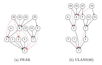
Figure 4.5: Main delivery paths of PEAR and ULANS(80). Dashed line indicates the unidirectional link between a pair of nodes.
