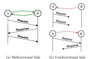
Figure 2.3: DTN node's information exchange when the link between node A and node B is bidirectional and unidirectional.
