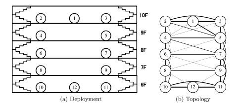
Figure 4.19: Configuration and topology of the experimented networks.
