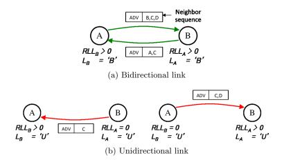
Figure 3.4: Example of reverse link lifetime (RLL) and link status (L) when the link between node A and node B is (a) bidirectional and (b) unidirectional.
