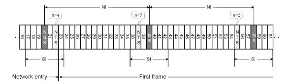
Fig. 5 First frame of STDMA
