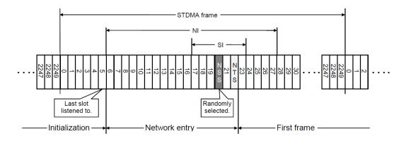
Fig. 4 Network entry of STDMA
