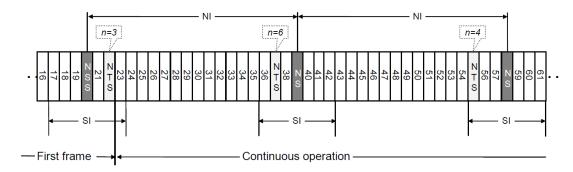
Fig. 6 Continuous operation of STDMA
