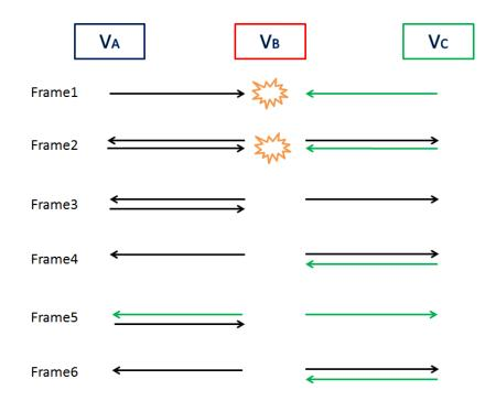
Fig. 12 the mechanism of TSS in three vehicles where STI<sub>A</sub>>STI<sub>C</sub> (colors represent the STIs of different vehicles)
