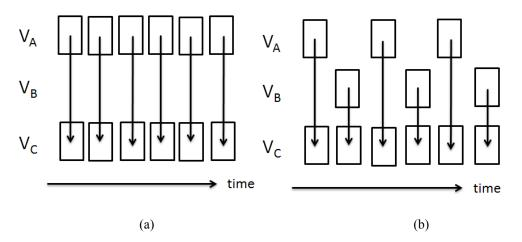
Fig. 11 Example of continuous blockings (a) and ideal timeslot usage (b)
