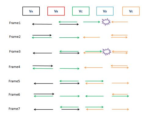
Fig. 14 the mechanism of TSS in five vehicles where  $STI_A \leq STI_E$  (colors represent the STIs of different vehicles)
