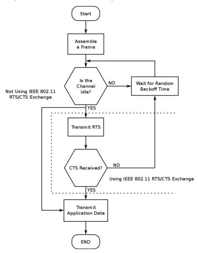
Fig. 2 Mechanism of CSMA/CA (http://en.wikipedia.org/wiki/Carrier sense multiple access with collision avoidance)
