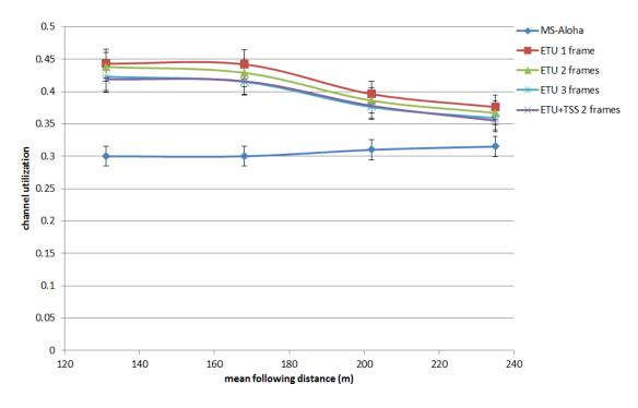
Fig. 27 Channel utilizations of different protocols in Scenario 2
