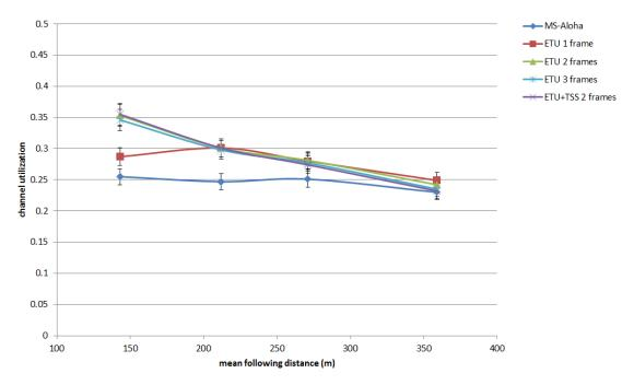
Fig. 23 Channel utilizations of different protocols in Scenario 1
