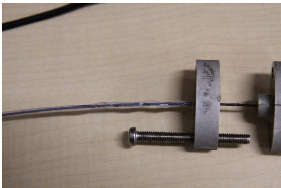
Fig. 7. 7 Deformed Teflon Tube
