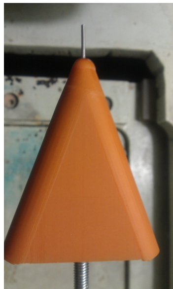
[Figure 2.14. Lifting-body model with flat-nose spike and l/D=1.5 .]
