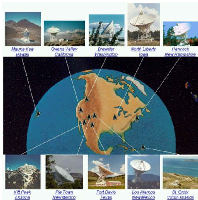
Figure 2.13: VLBA is a system of ten radio-telescope antennas, each with a dish 25 meters in diameter. Image Credit: NRAO.
