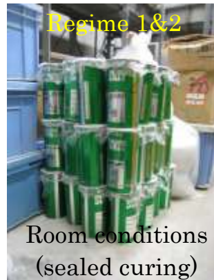
Figure 3.11 Sealed curing in room condition and hot water of 40°C curing
