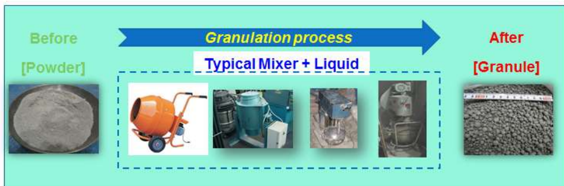
Figure 3.8 Principle of proposed granulation technique
