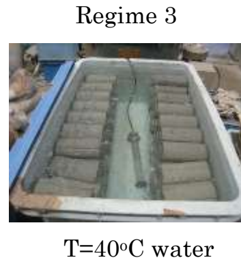
Figure 3.11 Sealed curing in room condition and hot water of 40°C curing
