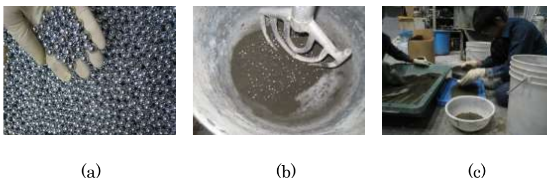
Figure 5.6 (a) Steel balls; (b) Mixing self-healing materials with steel balls; (c) Sieving process
