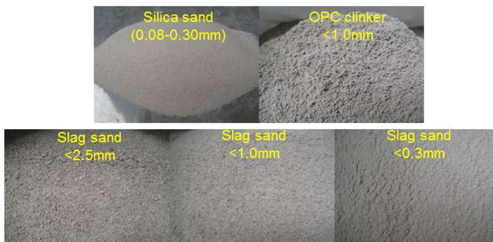
Figure 5.7 Different types of fine sand having certain healing capability
