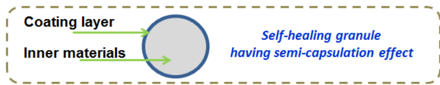
Figure 5.3 Two basic components of self-healing granule
