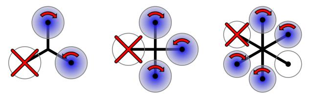
Figure 1: A failed propeller in the case of a tricopter, hexacopter, and hexacopter.
