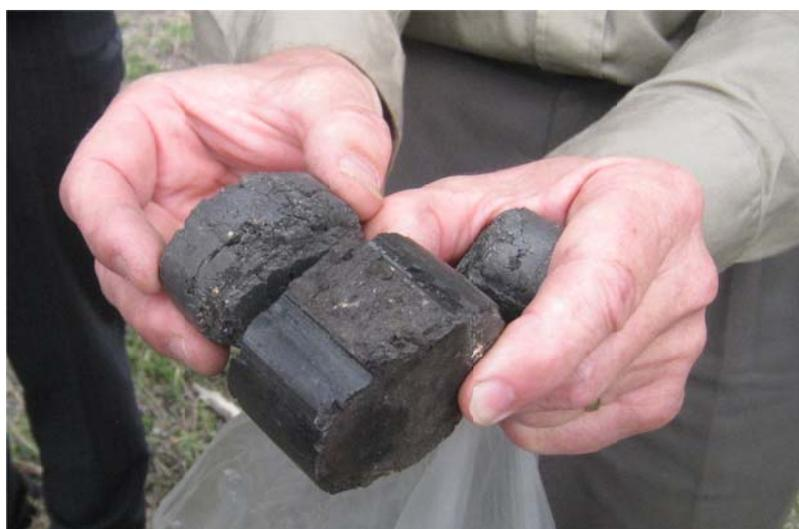
Fig. 1-8 Briquette made from Victorian lignite.
