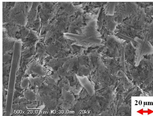
Figure 4.29 The SEM image of TiS 3 . The average width is around ca. 10 μm.
