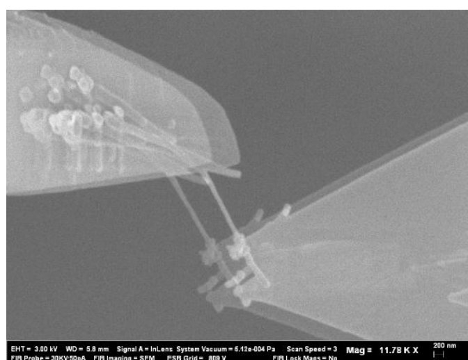
Fig.4.4 Problems for estimating young's modulus of CNT. CNT could not be pulled straightly.
