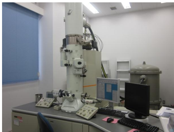
Fig.5.5 Transmission Electron Microscope used in this research (JEM-2100F, JEOL, Japan).
