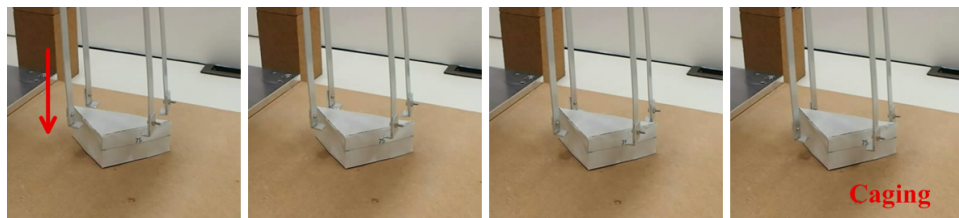
(a) The target object can be successfully caged with the implementation based on the simplified design and the robust caging algorithms
