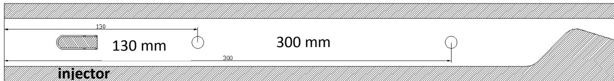
Figure 9 Schematic of the combustor using two thermocouples
