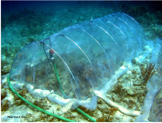
Figure 1-7. “SHARQ” (the Submersible Habitat for Analyzing Reef Quality) chamber system: Yates and Halley (2003, 2006) established “SHARQ” chamber system. “SHARQ” is a large, 4.9 (l) x 2.4 (w) x 1.2 (h)-meter, portable benthic incubation chamber designed to isolate a mass of water over the underlying substrate. A flow through analytical system enables continuous, 24-h monitoring of water chemistry resulting from benthic community processes. They conducted 24-h chamber experiments at Molokai reef, Hawaii. These pictures are cited from http://gulfsfci.usgs.gov/tampabay/reports/
