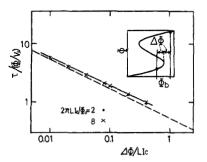
Fig. 3. Switching delay versus overdrive for the interferometer of Fig. 1(a). Solid line: numerical calculations. Dashed line: (4). Equation (4) agrees with the numerical calculation of (3) within about 15 percent for overdrives  $\Delta \Phi/LI_c$  below about 20 percent, and for values of  $LI_c$  ranging from about  $0.3\Phi_0$  to  $1.3\Phi_0$ .
