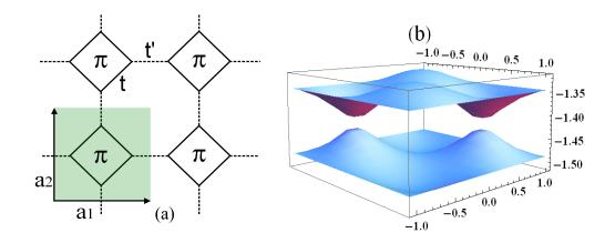
Figure 7.1: Figure 7.1(a) is  $\pi$ -flux octagon-square lattice, and Figure 7.1(b) is the plot of lowest two bands of Hamiltonian (7.1) with t = 1, t' = 0.1.
