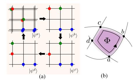
Figure 5.3: A schematic figure to explain the relation between original manybody problem and the tight binding model on a fictitious lattice. Figure 5.3 (a) demonstrates the process to exchange two particles in real lattice. Figure 5.3 (b) shows the corresponding loop in a fictitious lattice, where site *a* is identified with the many-body basis state  $|\psi^a\rangle$ . The flux  $\Phi$  in Fig. 5.3 (b) is  $\pi$  for fermions but zero for bosons.
