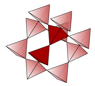
Figure 7.8: The lattice structure of pyrochlore. A dimer of two tetrahedra made up of 7 sites are shown in dark in pyrochlore lattice.
