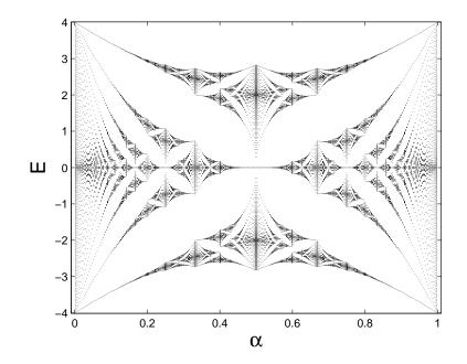
Figure 2.1: Hofstadter's butterfly: the energy spectrum of single electron on a two-dimensional square lattice in a uniform magnetic field, which is perpendicular to the lattice. Vertical variable is energy E and horizontal variable is flux density per plaquette  $\alpha$ , whose value is given by the number of flux quanta per plaquette  $\Phi/\Phi_0$ .
