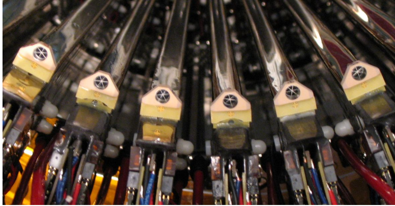
Figure 4.5: Corner cubes mounted on the downstream side of the drift chambers.
