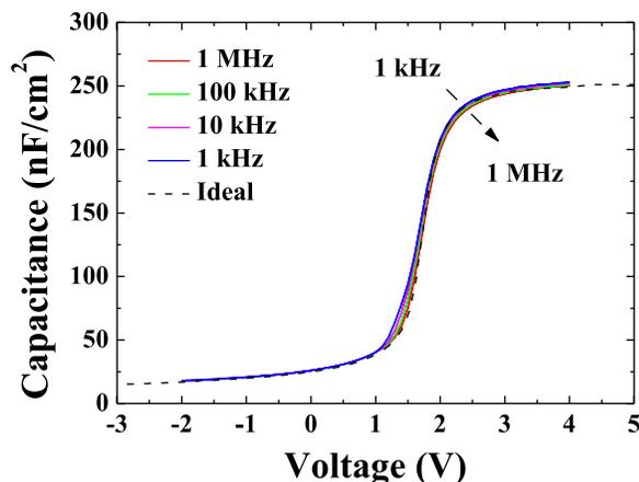
FIG. 1. Bidirectional C-V characteristics of the MOS capacitor ( $T_{ox} \sim 14 \text{ nm}$ ) fabricated by 1300 °C oxidation followed by POA at 800 °C in O<sub>2</sub>. Measurement was conducted at various frequencies from 1 kHz to 1 MHz. Broken line shows the ideal C-V curve calculated by Poisson's equation.
