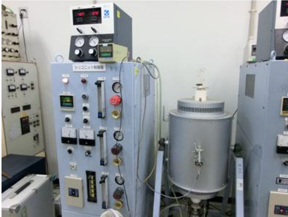
Fig. 3.6 Photograph of the furnace system. Left: temperature controller. Right: SILICONIT furnace with a gas mixing system.
