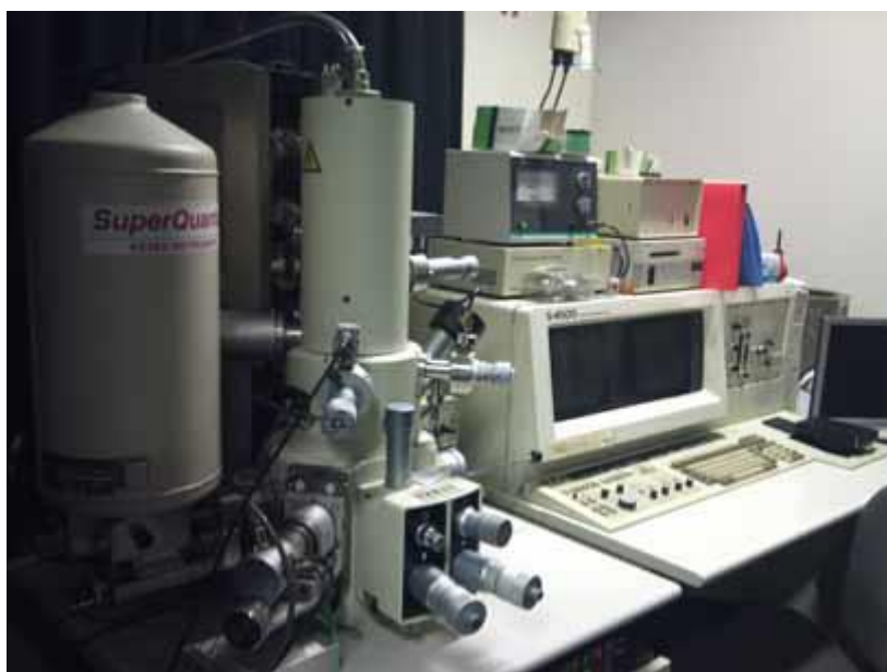
Fig. 3.1 FEG-SEM (Hitachi S-4500) at Department of Earth and Planetary Science, University of Tokyo.
