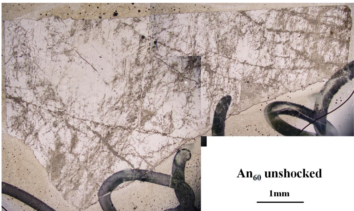
Fig. 2.55 Optical photomicrograph of An 60 unshocked sample (plane-polarized light).
