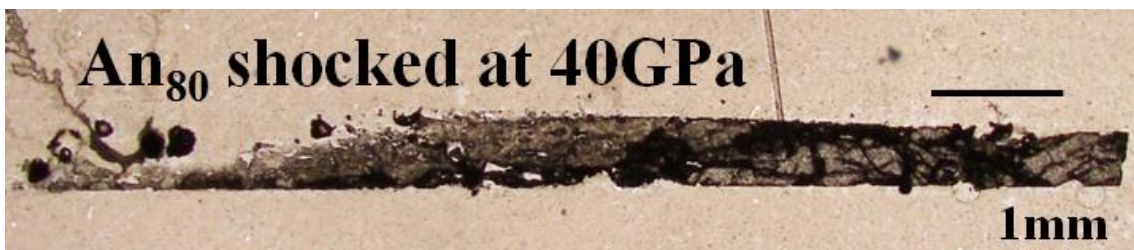
Fig. 2.54 Optical photomicrograph of An 80 plagioclase shocked at 40 GPa (plane-polarized light).
