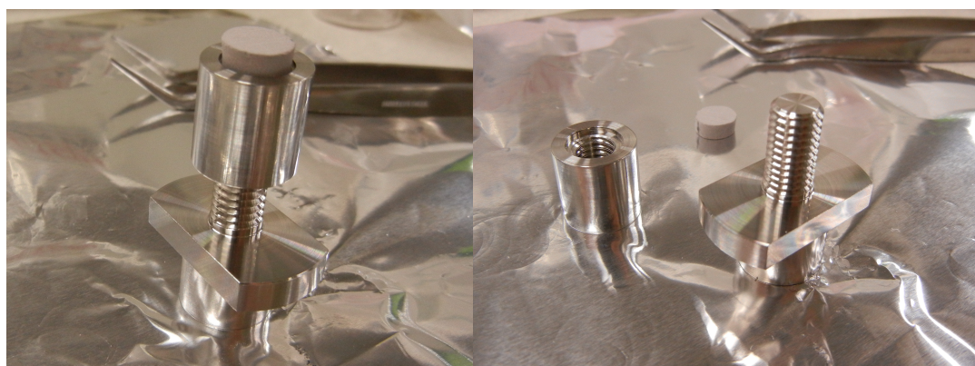
Figure 6.5 Sample holder and a pellet sample. The vertical position of the sample surface is adjustable. Each part is made of the stainless steel. For a scale, the diameter of the pellet sample is \sim 10 mm.
