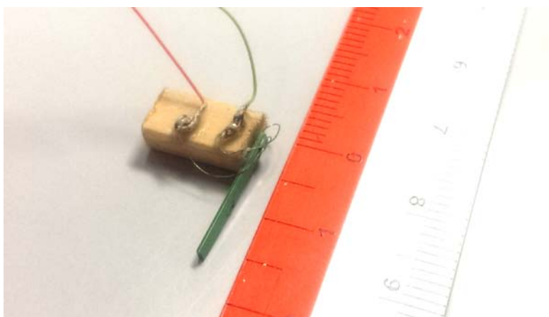
(b) Completed piezo-beam receiver assembly
