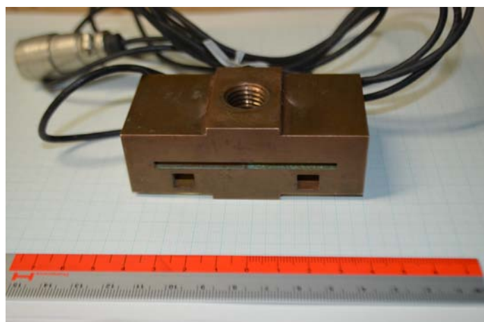
Figure 3.5: Axial load cell employed for this study.
