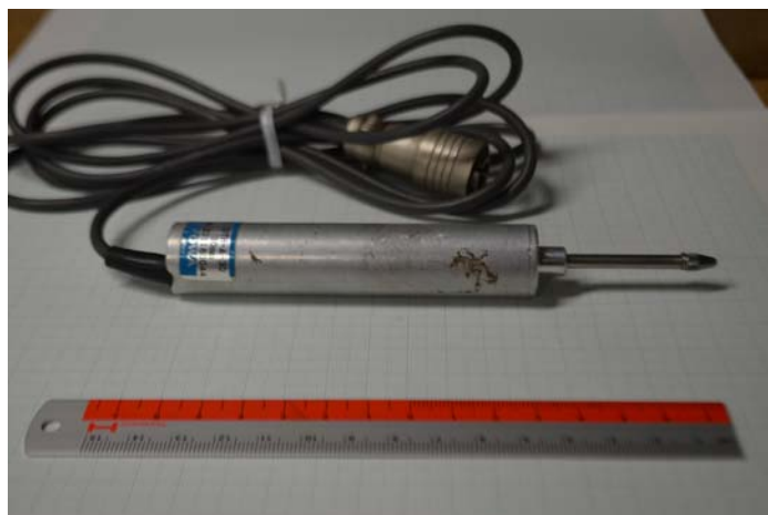
Figure 3.7: LVDT used in present study (0-30mm range).
