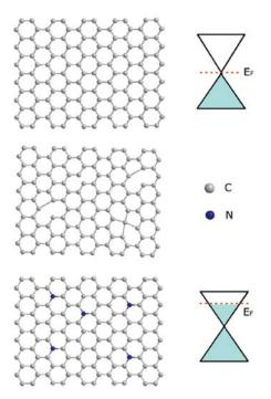
**Figure 1.19.** The atomic structure of graphene annealed in NH<sub>3</sub> after irradiation. Graphene is doped by substituting C atoms with N atoms.<sup>58</sup> Reproduced with permission. Copyright 2010, American Chemical Society.
