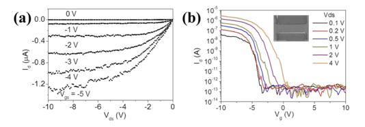
**Figure 3.27.** Electrical properties of 20 % acetonitrile induced HASWNT devices ( $L_c$ : 7  $\mu$ m and W: 20  $\mu$ m). (a) Output characteristics with V<sub>ds</sub> sweep from 0 to 10 V. (b) Transfer characteristics at various drain voltage. V<sub>GS</sub> was applied from -10 to 10 V with a 200 mV step in both cases.
