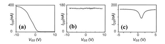
Figure 1.13. Drain current ( $I_{ds}$ ) as a function of the gate voltage ( $V_{gs}$ ) for a (a) semiconducting, (b) metallic, and (c) semiconducting with a small band gap SWNT.  $V_{ds} = 10 \text{ mV}$  for all data.<sup>6</sup>
