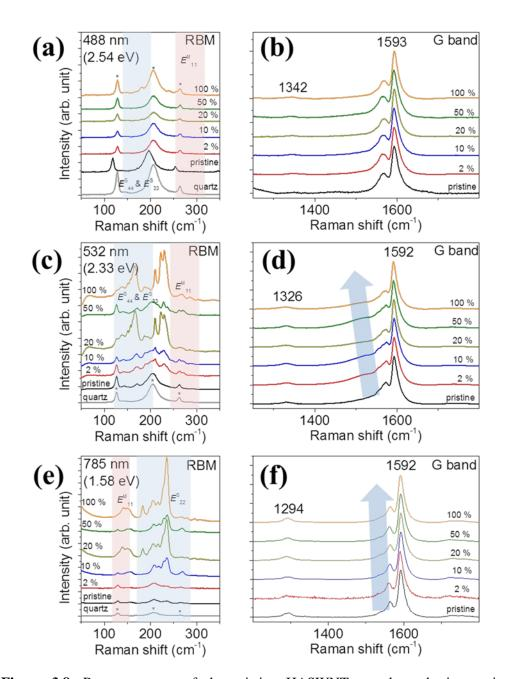
**Figure 3.8.** Raman spectra of the pristine HASWNT sample and nitrogen-induced HASWNT on an r-cut crystal quartz substrate at excitation energies of (a)-(b) 2.54 eV, (c)-(d) 2.33 eV, and (e)-(f) 1.58 eV. All Raman spectra were normalized to the G band intensity. The peaks marked by asterisks originated from the quartz substrates in RBM modes. The arrow shows the G band peak position shift in G band modes.
