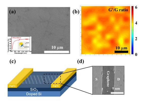
**Figure 2.6.** (a) SEM image for as-grown graphene on copper substrate via ACCVD. (b) Intensity ratio of G' to G band of scanning Raman spectroscopy using an excitation energy of 514.5 nm (2.41 eV). (c) The schematic of as-grown graphene field-effect transistors with source, drain, and gate electrodes. A 600 nm SiO<sub>2</sub> was used as an insulator layer. (d) The corresponding SEM image of graphene on silicon substrate between the source/drain electrodes after transferred.
