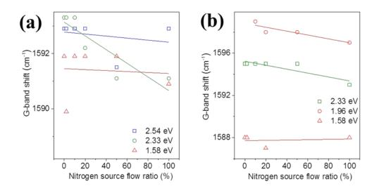
**Figure 3.12.** (a) G band peak shift of HASWNT on quartz substrates with an acetonitrile concentration increases. (b) G band peak shift of HASWNT on silicon substrates with an acetonitrile concentration increases.
