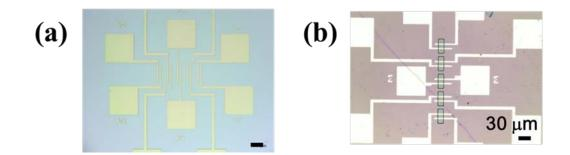
**Figure 2.3.** Optical micrograph of fabricated device array. (a) Optical image after first photolithography process. (b) Optical image after second photolithography process.
