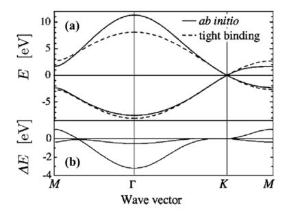
**Figure 1.5.** (a) Energy dispersion of graphene calculated by first principle (solid lines) and nearest neighbor tight-binding method as in this chapter (dashed lines). (b) Difference between the energy dispersions calculated in (a).<sup>11</sup> Reproduced with permission. Copyright 2002, American Physical Society.
