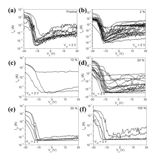
**Figure 3.16.** Corresponding transfer characteristics in terms of each device under vacuum condition (~10<sup>-3</sup>-10<sup>-4</sup> Pa), respectively ( $V_{ds} = 2$  V). (a) pristine, (b) 2 % acetonitrile concentration, (c) 10 %, (d) 20 %, (e) 50 %, and (f) 100 % HASWNT FETs.
