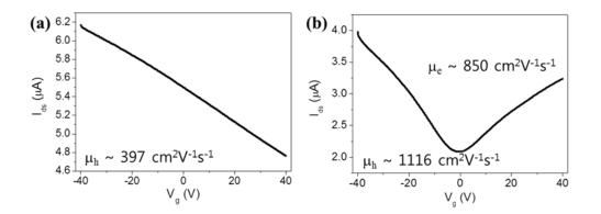
**Figure 2.17.**  $I_d$ - $V_g$  characteristics before and after PVA-10W coated graphene devices under ambient conditions ( $V_{ds} = -10 \text{ mV}$ ). (a) Transfer curve for as-grown CVD graphene transistor. (b) Transfer curve for PVA-10W coated graphene devices under ambient air condition.
