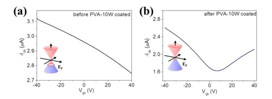
**Figure 2.10.** Electronic transport properties of as-grown ACCVD graphene devices. (a) Transfer characteristics before PVA-coated graphene device under ambient condition (Channel length = 10  $\mu$ m; width = 10  $\mu$ m; V<sub>ds</sub> = -10 mV). (b) Transfer characteristics after PVA-10W coated ACCVD graphene transistors in air.
