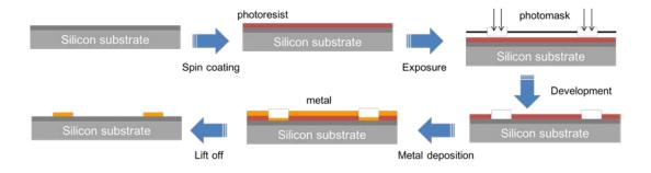
Figure 2.4. Process steps for graphene-FET fabrication.
