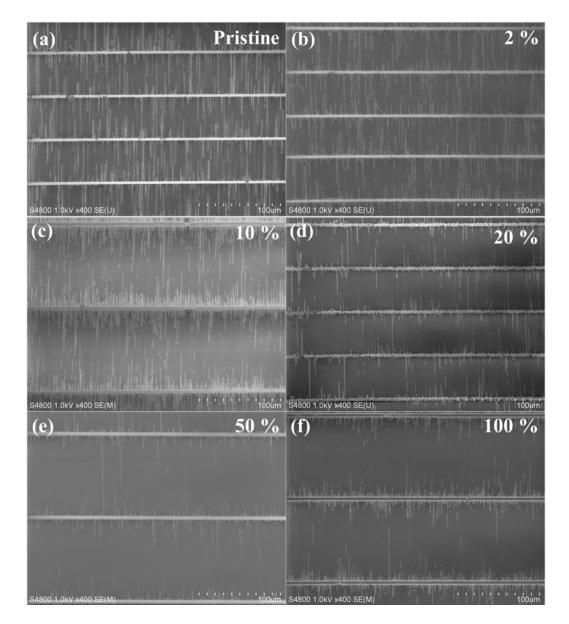
**Figure 3.7.** SEM images of nitrogen-induced HASWNTs and ethanol-based HASWNTs on a quartz substrate by CVD growth as a function of acetonitrile concentration , for instance, (a) low density pristine, (b) 2 %, (c) 10 %, (d) 20 %, (e) 50 %, and (f) 100 %, respectively. (Scale bars are 100 μm)
