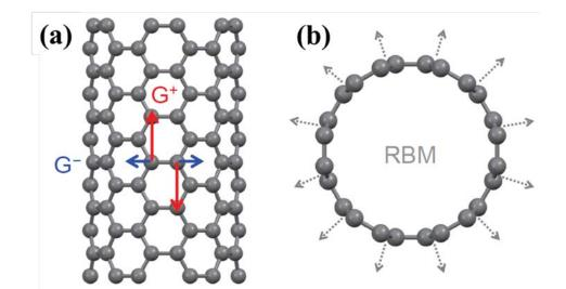
**Figure 1.10.** (a) The in-plane vibrational modes corresponding to the G-band Raman signal, and (b) the uniform out-of-plane vibration that gives rise to the radial breathing mode excitations.
