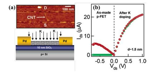
**Figure 1.15.** n-doping of nanotubes by K vapor. (a) AFM image of a nanotube device (top) and schematic drawing of K doping of the device (bottom). (b)  $I_{ds}$ - $V_{ds}$  chracterisitics of a device before and after K doping at two gate voltage  $V_{gs} = -3$  (red) and 0 V (green).<sup>42</sup> Reproduced with permission. Copyright 2005, American Chemical Society.
