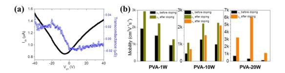
**Figure 2.18.** (a)  $I_{ds}$ - $V_{gs}$  characteristics and transconductance as a function of gate voltage for PVA-10W doped graphene transistors ( $V_{ds} = -10 \text{ mV}$ ). (b) Hole and electron mobility before and after PVA-1W, -10W, and -20W coated graphene devices as a function of different channel widths, respectively.
