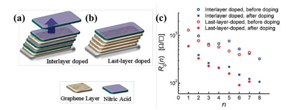
**Figure 1.20.** Schematic of (a) interlayer doped and (b) last-layer doped graphene stacks. (c) Sheet resistance versus number of layers for both interlayer and last-layer doped cases.<sup>60</sup> Reproduced with permission. Copyright 2010, American Chemical Society.
