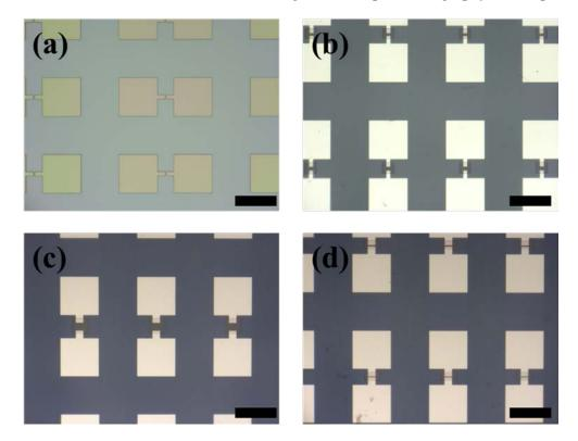
**Figure 3.4.** Optical images of patterning HASWNTs on SiO<sub>2</sub>/Si and PET substrates after 1st and 2nd photolithography procedures, respectively. (a) and (b) are on a silicon substrates. (c) and (d) is optical images in PET substrates. (Scale bars are 100  $\mu$ m)
