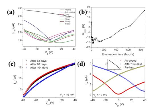
**Figure 2.19.** (a) Transfer curves of PVA-10W doped graphene FETs as a function of time. (b) Dirac point of PVA-10W GFET as a function of evaluation time. (c) I-V characteristics of as-grown, PVA-20W doped, after 104 days, and re-heat treatment graphene devices, respectively. (d)  $I_{ds}$ -V<sub>gs</sub> characteristics of PVA-10W doped, after 104 days, and re-heat treatment graphene FETs (that of the as-grown graphene device in inset).
