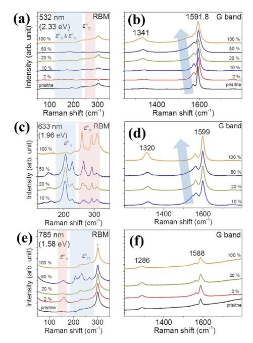
**Figure 3.9.** Raman spectra at various excitation energies of the HASWNT and N-HASWNT samples on SiO<sub>2</sub>/Si: (a) and (b) 2.33 eV, (c) and (d) 1.96 eV, and (e) and (f) 1.58 eV. All Raman spectra were normalized to the G-band intensity. The numbers in each figure are the diameters of the corresponding peaks in nm and phonon frequencies.  $E^{S(M)}_{ii}$  indicate the van Hove singularity transition energy between the *i*th levels of the semiconducting (metallic) nanotube.
