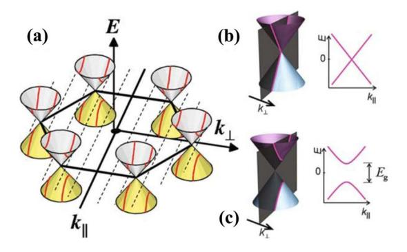
**Figure 1.7.** (a) A first Brillouin zone of graphene with conic energy dispersions at six **K** points. The allowed  $k_{\perp}$  states in a SWNT are presented by dashed lines. The band structure of a SWNT is obtained by cross-sections as indicated. Zoom-ups of the energy dispersion near one of the **K** points are schematically shown along with the cross-sections by allowed  $k_{\perp}$  states and resulting 1D energy dispersions for (b) a metallic SWNT and (c) a semiconducting SWNT.
