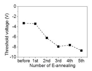
Figure 3.20. Threshold voltage shift as number of e-annealing increase with 20 % acetonitrile concentrations through  $I_d$ -V<sub>g</sub> curves in the linear region in vacuum condition.
