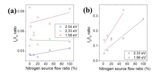
**Figure 3.13.** (a) Intensity ratio of D band to G band of HASWNT on quartz substrates with an acetonitrile concentration increases. (b) Intensity ratio of D band to G band of HASWNT on silicon substrates with an acetonitrile concentration increases.
