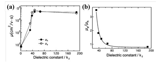
**Figure 1.18.** (a) Carrier mobility versus dielectric constant of solution ( $\kappa_2$ ). Both electron and hole mobility improve as  $\kappa_2$  increases. (b) Ratio of electron to hole mobility versus  $\kappa_2$ .<sup>57</sup> Reproduced with permission. Copyright 2009, American Chemical Society.
