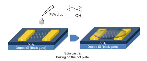
Figure 2.9. Process steps for PVA-coated graphene device.
