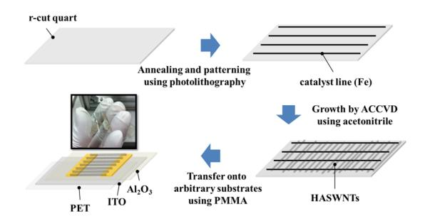
Figure 3.1. Growth procedures of horizontally aligned carbon nanotube on a quartz substrate.
