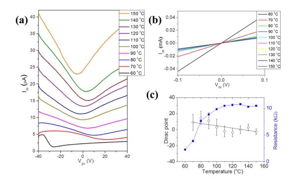
**Figure 2.12.** I-V characteristics of PVA-10W doped graphene transistors. (a) Corresponding  $I_{ds}$ - $V_{gs}$  characteristics of PVA-10W coated graphene devices as a function of different hardening temperature for 10 min. Drain current are shifted for clarity. (b) Dirac point position depends on diverse hardening temperature. (c) The corresponding  $I_{ds}$ - $V_{ds}$  characteristics as a function of different hardening temperature.
