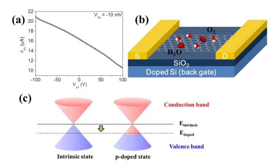
**Figure 2.8.** (a) Corresponding transfer  $(I_{ds}-V_{gs})$  characteristics of as-grown graphene device. (b) Water, oxygen, and/or residues adhere on graphene surface. (c) Schematic illustration of the Fermi level shift of monolayer graphene in air.
