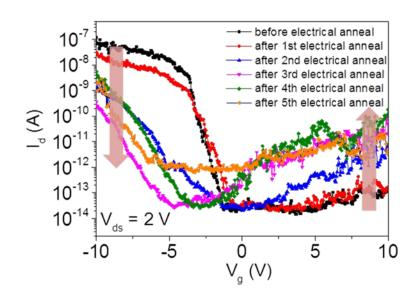
**Figure 3.18.** Corresponding  $I_d$ - $V_g$  characteristics of the 20 % N-HASWNT FETs before/after annealing using electrical annealing in vacuum condition (~  $10^{-3}$ - $10^{-4}$  Pa).
