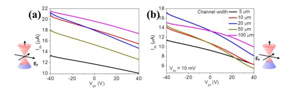
Figure 2.14. (a) Transfer curves of as-grown graphene transistors before PVA-1W doping.
