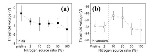
**Figure 3.19.** Threshold voltage shift as function of nitrogen-induced various acetonitrile concentrations ratio through transfer characteristics in the linear region. (a) In air. (b) In vacuum condition.
