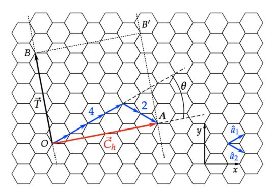
Figure 1.6. Representation of a SWNT by a chiral vector,  $\mathbf{C} = n_1 \mathbf{a}_1 + n_2 \mathbf{a}_2$ . In this figure, the wrapping index of the SWNT described by  $\mathbf{C}$  is (4,2).  $\mathbf{a}_1$  and  $\mathbf{a}_2$  are unit vectors of the underlying graphene lattice.
