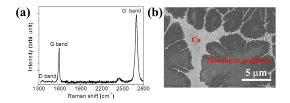
**Figure 2.7.** (a) Raman spectroscopy using an excitation energy of 488 nm (2.54 eV) for as-grown LPCVD graphene on SiO<sub>2</sub>/Si substrate. (b) Graphene domain grown at 1000 °C on Cu an average growth rate of ~ 50  $\mu$ m per 30 seconds.
