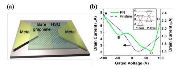
**Figure 1.22.** (a) Schematic of a graphene p-n junction—one half of the graphene surface is doped p-type and the other half is doped n-type by HSQ. (b) Electrical testing reveals a double dip for the p-n junction; the Fermi level separation is found to be more than 340 meV. <sup>69</sup> Reproduced with permission. Copyright 2010, American Physical Society.
