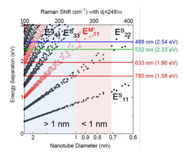
**Figure 3.10.** Kataura plot obtained from extended tight-binding model. The solid line is incident laser energies used in experiment.
