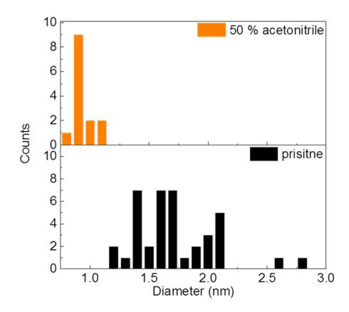
Figure 3.24. Comparison of the diameter distribution between pristine and 50 % N-HASWNTs. For pristine sample, mean diameter is  $\sim 1.7$  nm with standard deviation 0.4 nm. For 50 % N-HASWNT, mean diameter  $\sim < 1$  nm.
