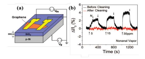
**Figure 1.17.** (a) Device schematic. (b) Measured sensor responses, before and after device cleaning. Exposure to nonanal vapor results in a 3 % change in current (for 5 ppm exposure) before sample cleaning; but the response drops by 1-2 orders of magnitude after sample cleaning.<sup>50</sup> Reproduced with permission. Copyright 2009, American Chemical Society.
