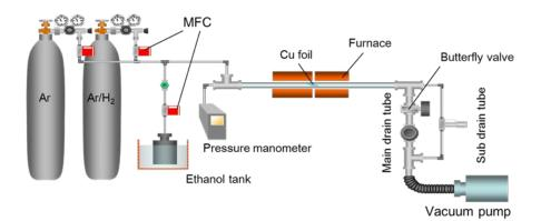
Figure 2.1. Schematic illustration of alcohol catalytic chemical vapor deposition.
