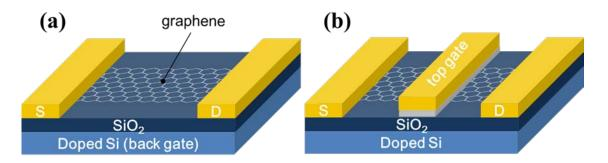
**Figure 1.14.** Back-gated and top-gated graphene FETs are shown in (a) and (b) respectively. Exfoliated and CVD graphene are usually on 300 nm or 90 nm SiO<sub>2</sub> substrate on doped Si. The doped Si allow for backgating.
