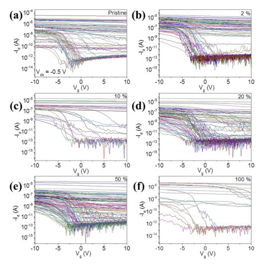
**Figure 3.15.** Corresponding transfer characteristics in terms of each device in ambient air condition ( $V_{ds} = -0.5$  V), respectively. (a) pristine, (b) 2 % acetonitrile concentration, (c) 10 %, (d) 20 %, (e) 50 %, and (f) 100 % HASWNT FETs.
