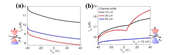
Figure 2.15. (a) Transfer curves of as-grown graphene devices before PVA-20W doping.(b) Transfer characteristics of PVA-20W doped graphene transistors as a function of gate voltage for varying channel widths.
