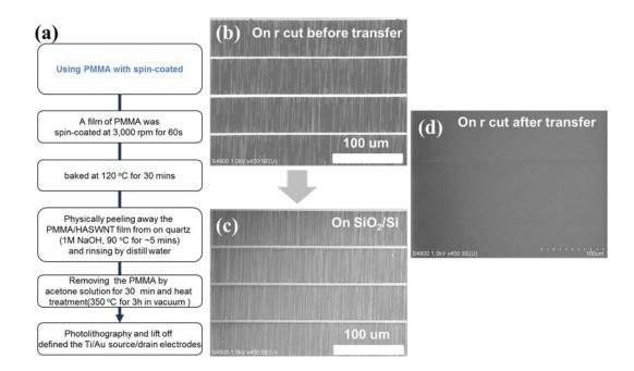
**Figure 3.3.** (a) Transfer process of HASWNTs on a quartz substrate. (b), (c), and (d) SEM images of HASWNTs on quartz and SiO<sub>2</sub>/Si substrates before/after transfer carbon nanotube by PMMA, respectively.
