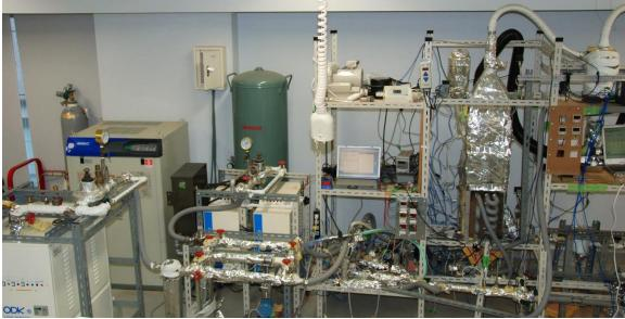
Fig. 5-3-1. Schematic diagram of an experimental fluidized bed dryer
