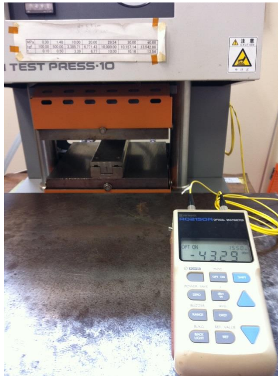
Fig. 4-11. An optical meter used to monitor the curing process
