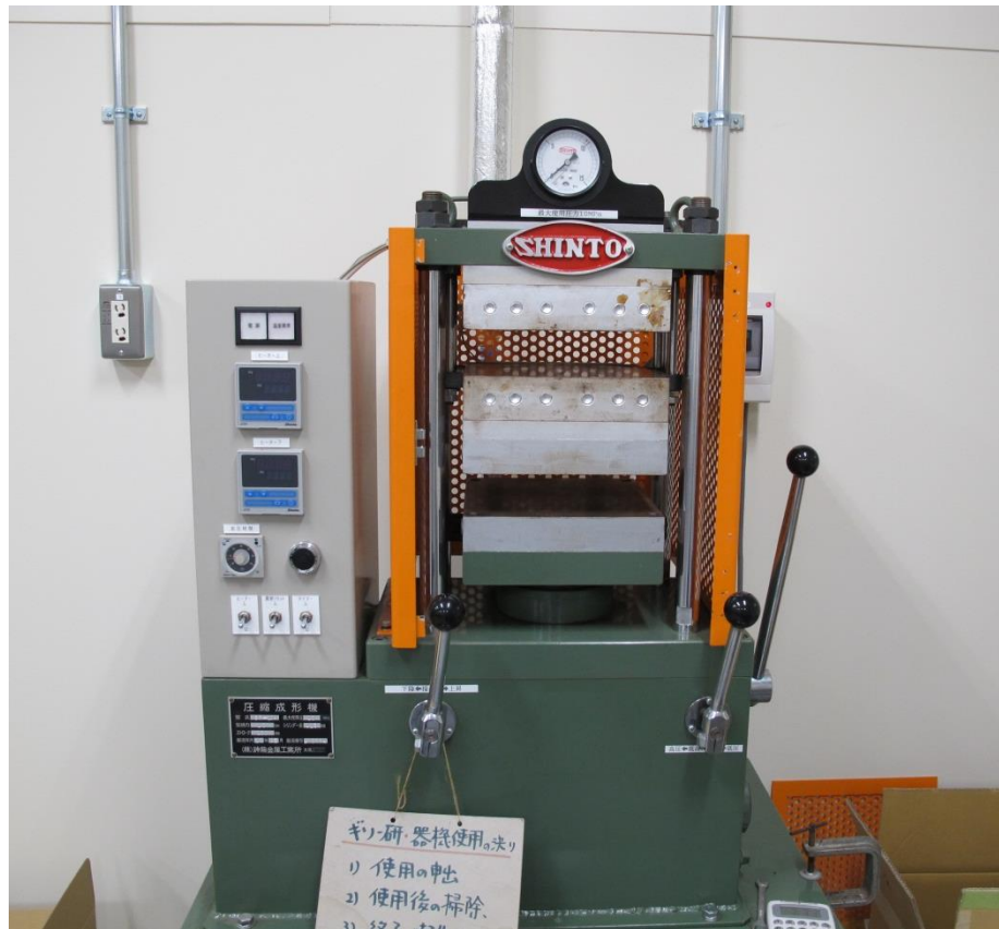
Fig. 4-16. Test press for joint bonding
