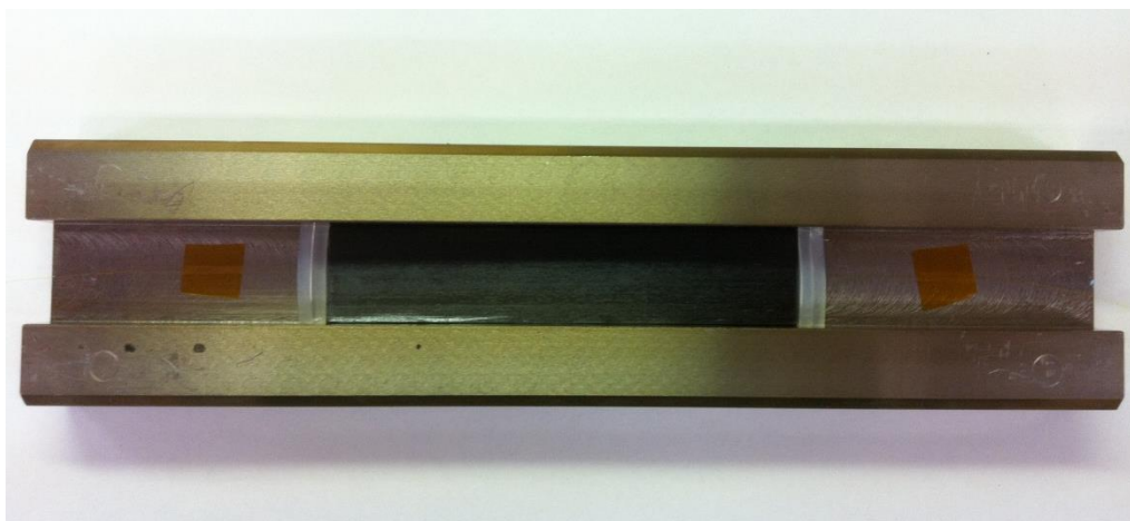
Fig. 4-6. The stacked CFRP prepregs upon the FBG in curing jig
