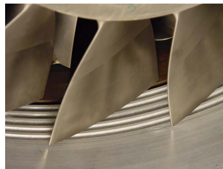
Figure 1.10 Typical application style of circumferentially grooved casing treatment [45]
