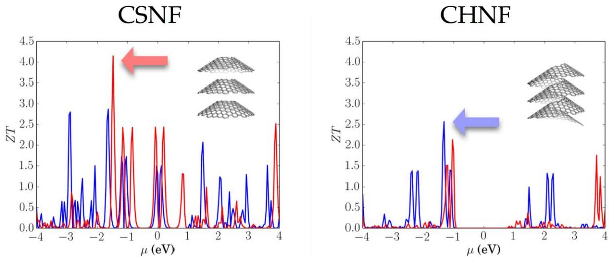
Fig. 3. Estimated thermoelectric figure of merit  $ZT$  for CSNF (left) and CHNF (right) nanostructures for (4,1,1) (blue) and wider radius (5,1,1) (red) configurations.
