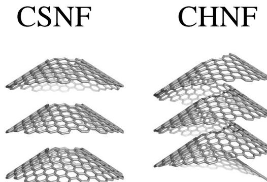
Fig 1. Conical nanofiber nanostructures investigated in this dissertation. The structures are the cup-stacked nanofiber (CSNF) and the conical-helix nanofiber (CHNF).
