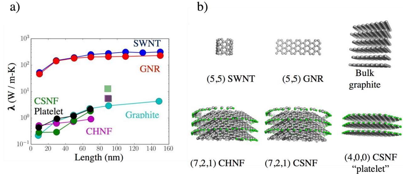
Fig. 2. Thermal conductivity calculated (a) for a variety of carbon nanostructures (b). The nanofiber thermal conductivity is two orders of magnitude lower than SWNT and GNR.
