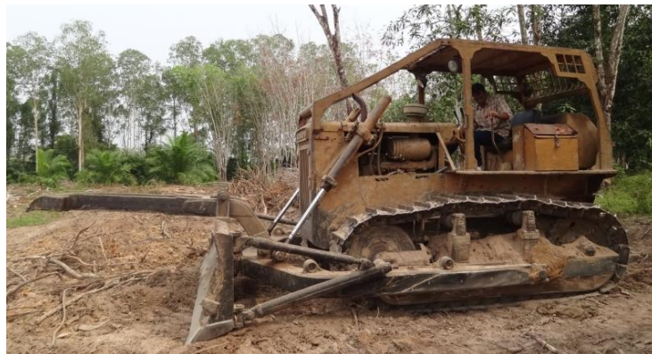
Figure 0.2 The modified bulldozer attached with tree pusher
