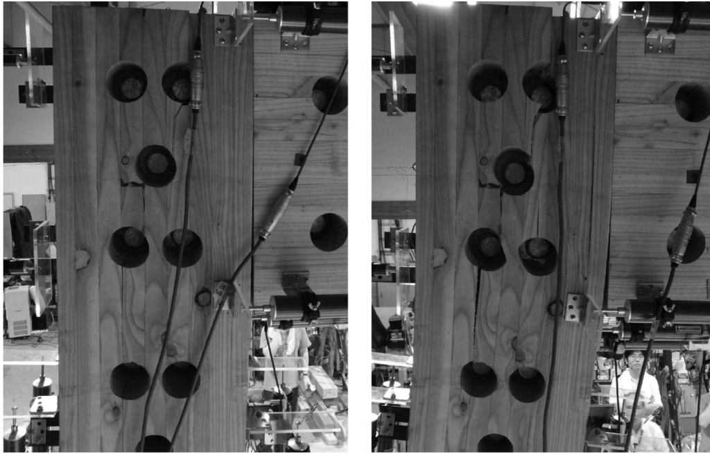
Fig. 3.31. Shear cracks at pre-drilled hole periphery
