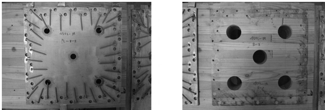
Fig. 3.25. Screws and screwed hole after test
