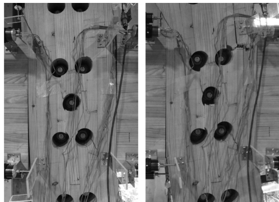
Fig. 3.65. Shear cracks at pre-drilled hole periphery
