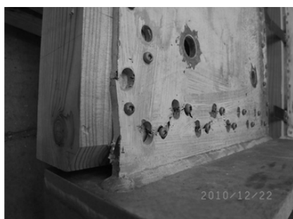
Fig. 4.14. Breaking line of steel
