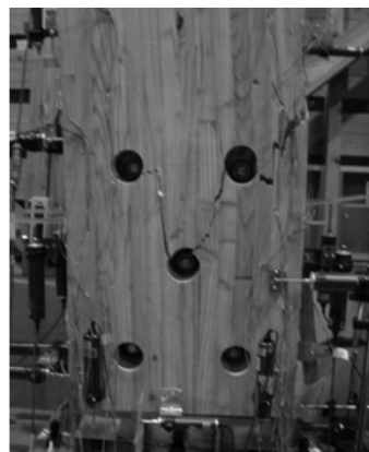
Fig. 4.13. Bending failure at joint end
