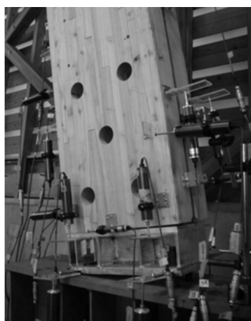
Fig. 4.15. Column-base joint at ultimate deformation of 450Ia at test
