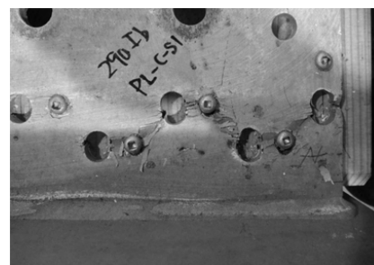
Fig. 4.18. Screwed holes after test
