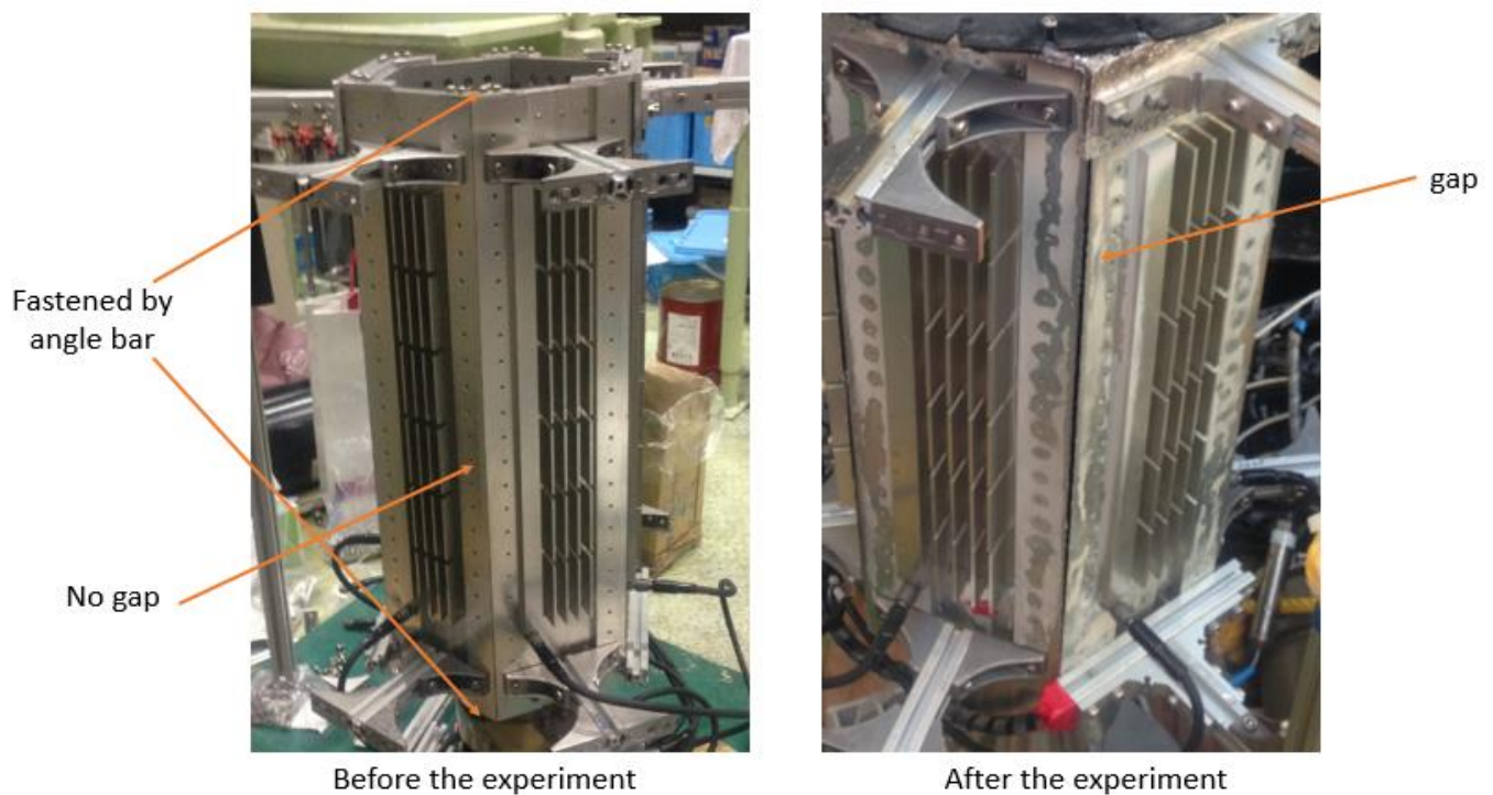
Fig. 5.27 The deformation of the structure
