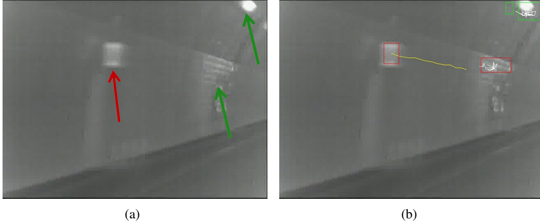
Figure 3.4: Original data and detection results. In (a), the red arrow points to the target object: emergency telephone indicator, and the green arrows point to noisy objects. In (b), red rectangles mark detection hypotheses labeled as positive using appearance information, and green rectangles mark negative ones. Yellow trajectories mark detection hypotheses labeled as positive using temporal information, and white trajectories mark negative ones.
