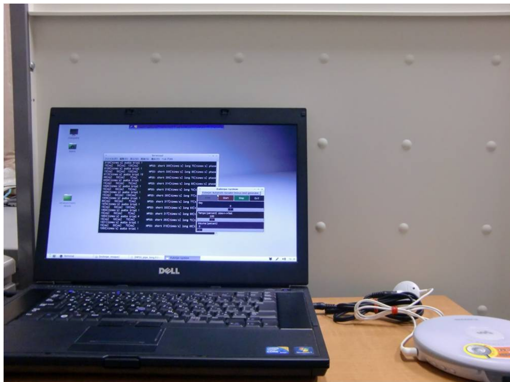
Figure 4.7:: Photograph of experiment system. There are a laptop PC, in which Euterpe system works, and CD player which is connected to the line input of the PC, from which an audio signal is input into the Euterpe system.
