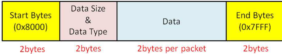
Fig. 4.7. Structure of packets from PC to MCU.
