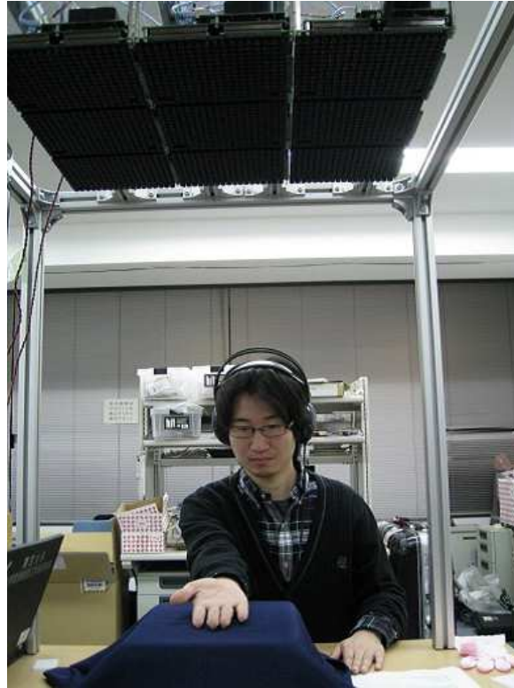
Fig. 4.18. Picture of the identification experiment. On the top of the cabinet was the 9-unit AUTD mounted.
