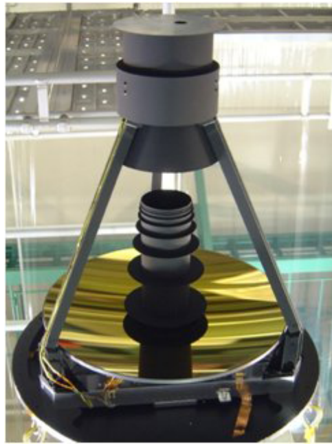
Figure 2.3 Picture of the AKARI telescope system. The mirrors are made of gold-coated silicon carbide.
