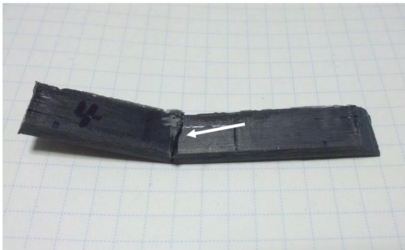
Figure 3.8 Specimen broken between loading points (specimen 4)
