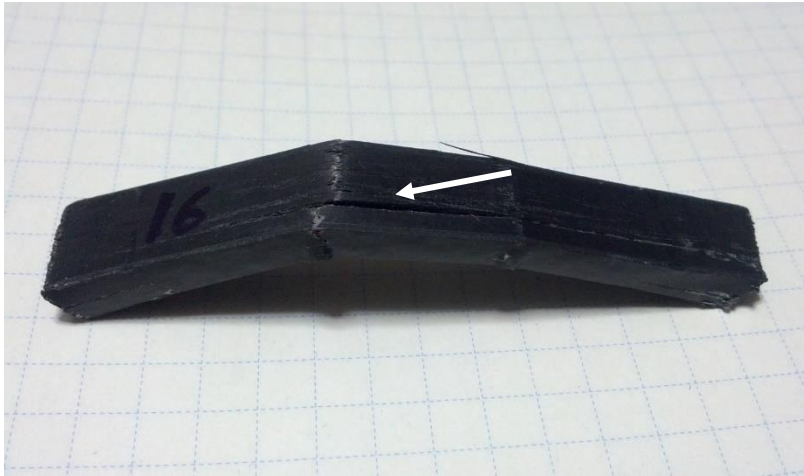
Figure 3.7 Split along the fiber direction (specimen 16)
