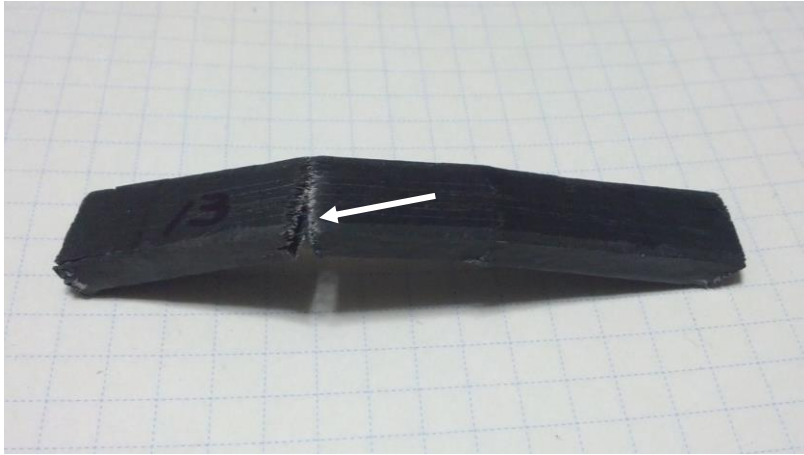
Figure 3.6 Specimen broken under loading points (specimen 13)
