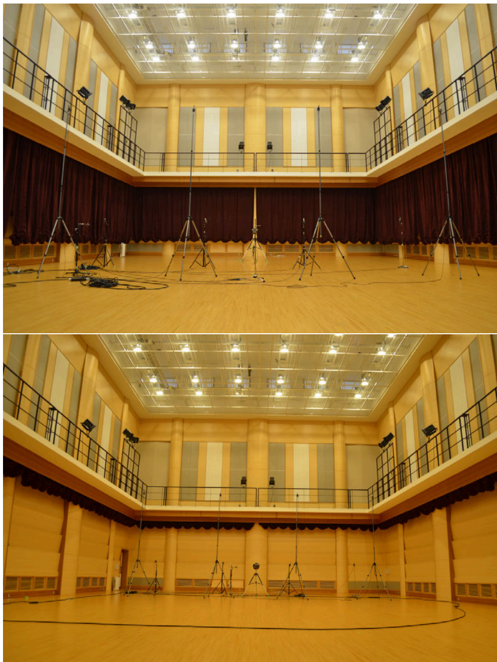
Fig. 2.5: Appearance of the impulse response measurement.
